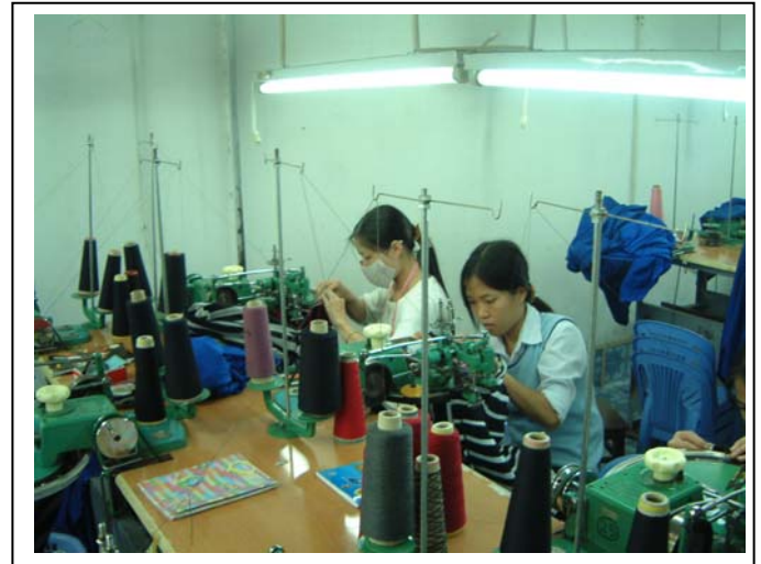
Figure 7: Avoid polished surfaces – use matt finishes or move the work position by 90 degrees to the right or left to stop reflected glare .
