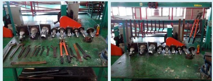
Tool racks were set up at the fitter's workstation. Tools are properly hanged and easy to reach. More space is available for operation. Abrasions between tools and molds are effectively reduced.
