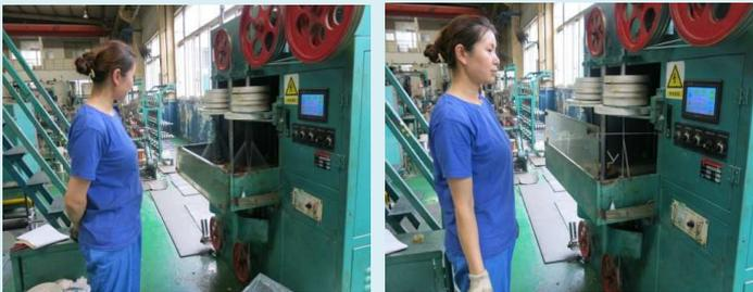
A protective shield was installed at the wrapping machine to prevent safety hazards of flying debris from the spinning parts.
