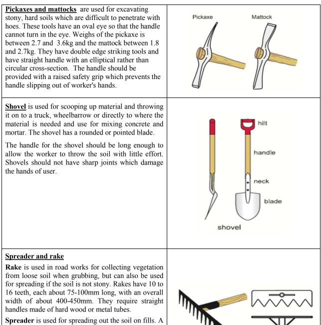
spreader is used for spreading out the solit off fins. A spreader can be a heavy-duty rake. The spreader is very useful when forming the camber and for spreading gravel. It is made of sheet metal (3-4mm thick) and have a ridge for crushing lumps of soil. Spreader can be pointed or flat, depending upon the nature of the gravel to be spread.
