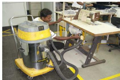
Do not sweep or use compressed air to clean machines - use an industrial vacuum.
