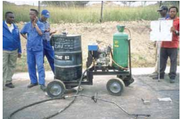
Example of a motorized hand sprayer
