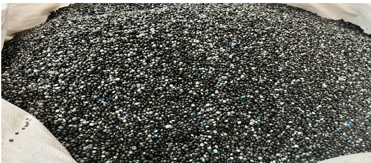
Photo 5.7 Plastic irrigation pipes are broken down for granulation
