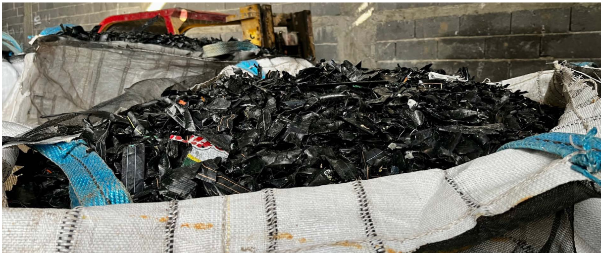
Photo 5.6 Plastic irrigation pipes are broken down into small pieces called “çapak”
