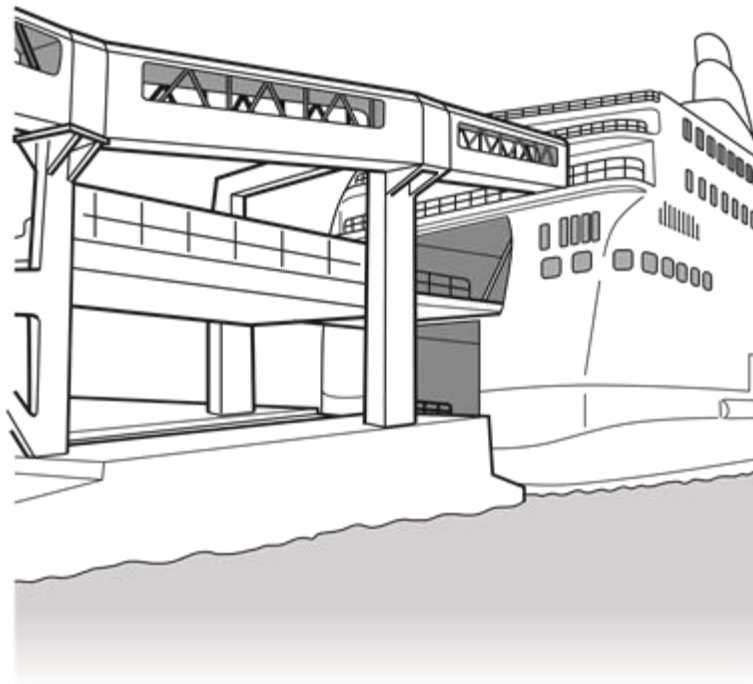
Figure 11. Linkspans and walkways
