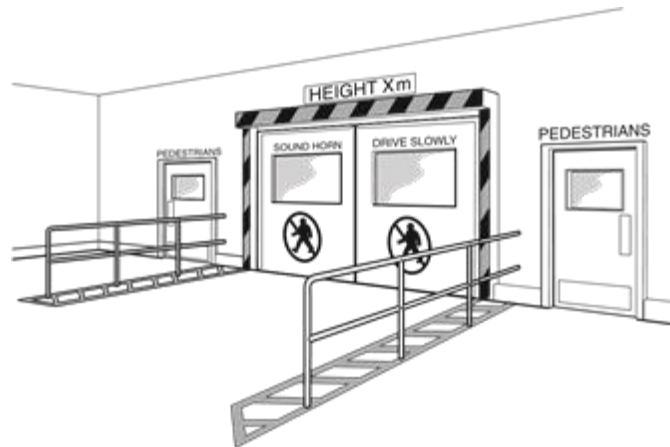
Figure 4. Low doorway markings with maximum heights
