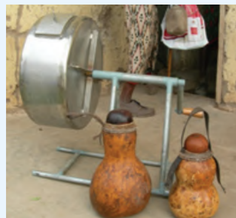
Photo 2. Improved aluminium manual butter churn
