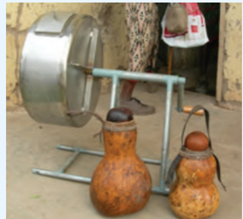
Photo 2. Improved aluminium manual butter churn
