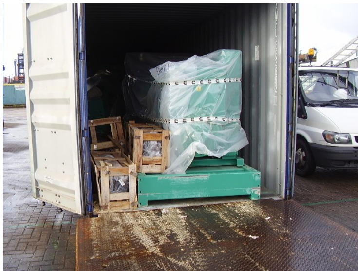
Figure 4.1. Chargement mal arrimé
