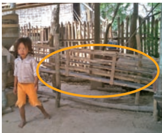
Figure 6-4. Father covered a moving belt of a rice-milling machine to protect his daughter from machine accidents
