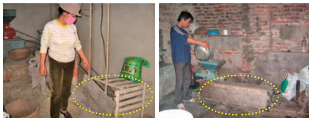
Figure 5-8. Covering moving machine belts.
