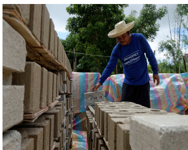
ICEB are more durable than traditional concrete blocks.
