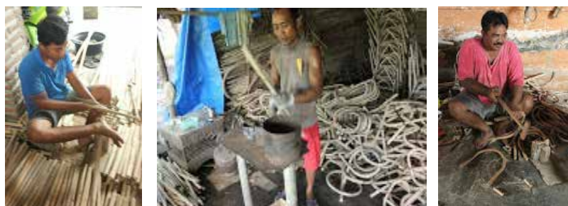
Cutting and bending the rattan for chair frames
