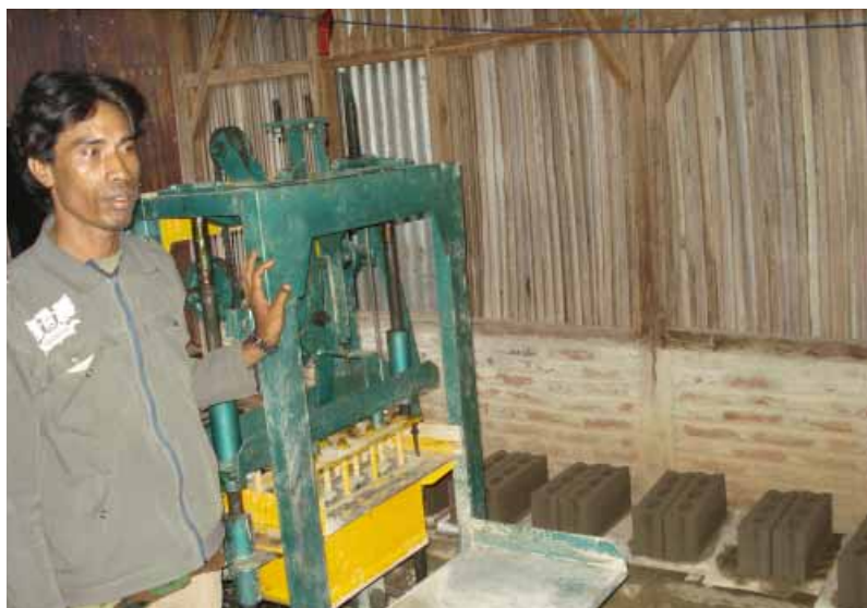
Figure 29: Youth group making cement building blocks
