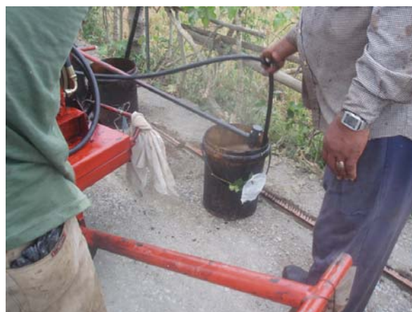
Picture 1: cleaning of emulsion sprayer after use
