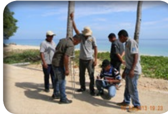
Reading the depth of penetration of the DCP cone Lee didiak penetrasaun cone husi instrumentu DCP
