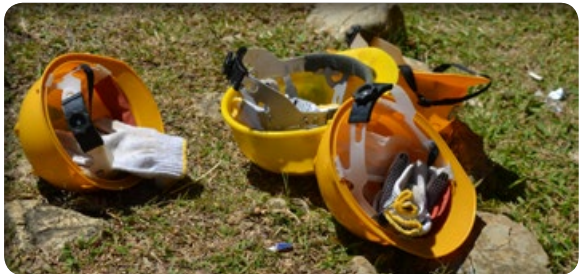
Safety hats are used if there is a risk that materials could fall down Sapeo sigur uza wainhira iha risku material bele monu tan ba ema
