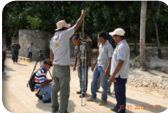
Training on DCP testing for MFW staff and local contractors Formassaun kore-ba teste DCP ba pessoal MOP sira no kontrator lokal sira
