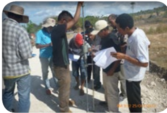
Showing how the penetration of the cone should be measured Hatudu onsa presiza sukat penetrasaun cone
