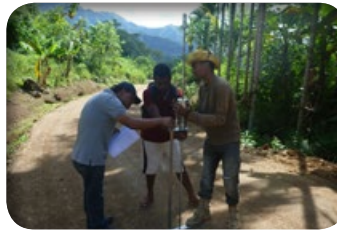
DCP readings are taken at regular intervals Lee DCP sei halo iha intervalu regular
