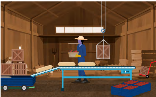
► Figure 6d. Short conveyors at different heights for loading or unloading materials
