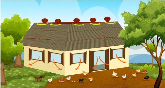
► Figure 17a. Open door and unobstructed windows to improve natural ventilation
