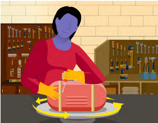
► Figure 10c. Rotating table to minimize the manual movement of heavy objects
