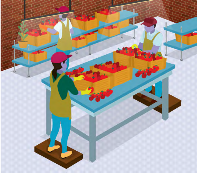
► Figure 7a. Foot platforms adjust the work height of shorter workers to elbow level
