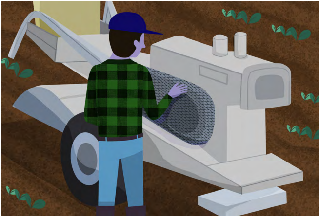
► Figure 13a. Safety guard made of locally available materials. For example, using a metal mesh allows you to observe the operation safely
