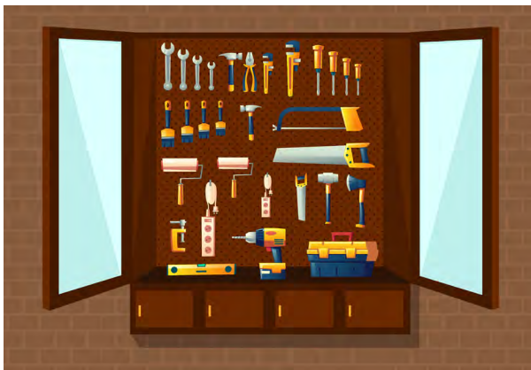
► Figure 3b. A cabinet for tools: pliers, hammers, saws, etc., should be hung neatly on both sides and with the edges facing the wall, in clearly labelled locations
