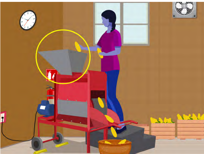
► Figure 14b. Feeding the hopper from a platform to improve the work height and allow good posture
