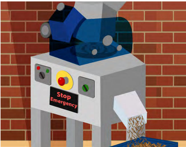
► Figure 15b. Red emergency stop button on the control panel clearly labelled, large and easily visible and readable
