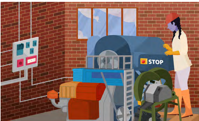
► Figure 16b. Electrical cables, control panel and switches properly secured to the wall, covered and lined
