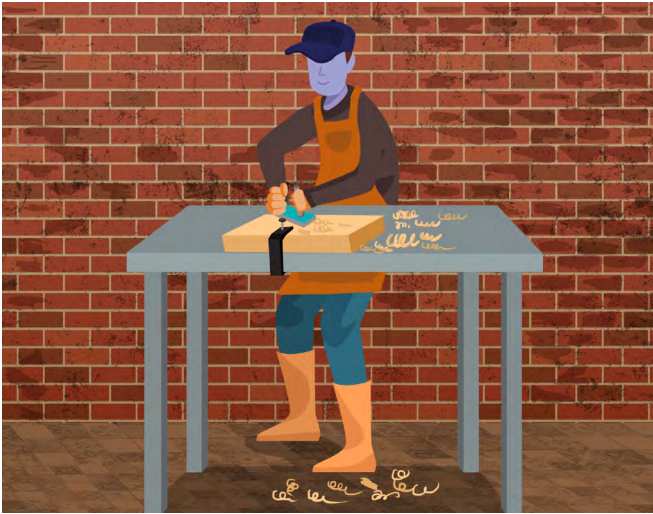
► Figure 11a. Using a piece of wood as a clamp during planing is a low-cost alternative
