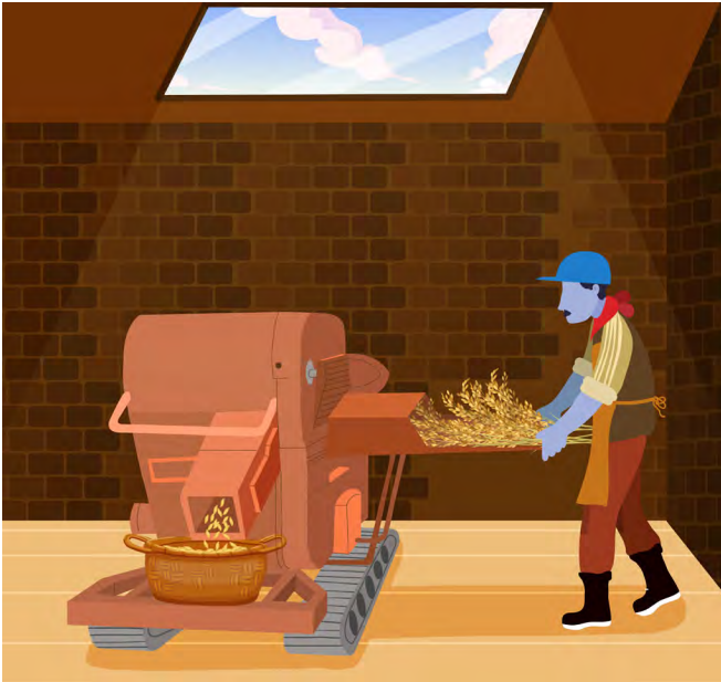
► Figure 14a. Feeding device connected to a threshing machine that gradually takes in rice bundles and separates the grains
