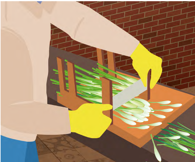
► Figure 11b. Simple clamping for easy and safe cutting work ensures product consistency
