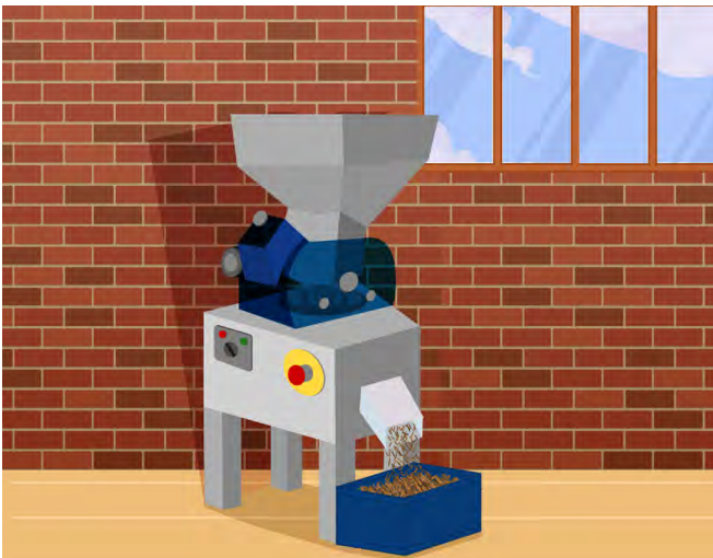
► Figure 14c. Funnel-type feeding device for milling
