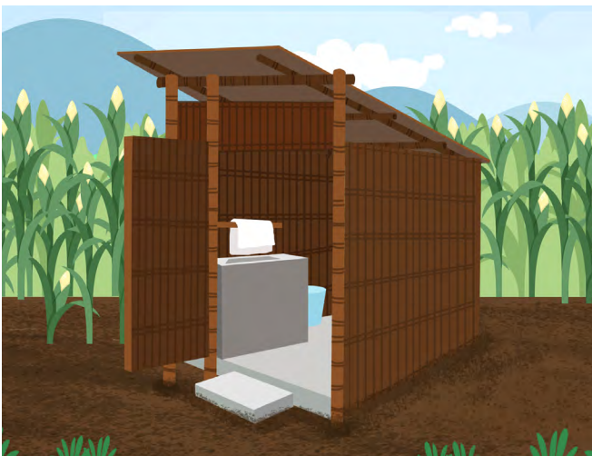
► Figure 26b. Latrine-type bathroom made from locally available materials
