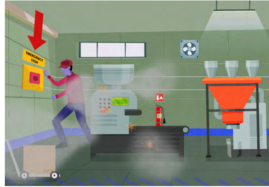
► Figure 15a. Red emergency stop button – large and clearly visible and easy to reach
