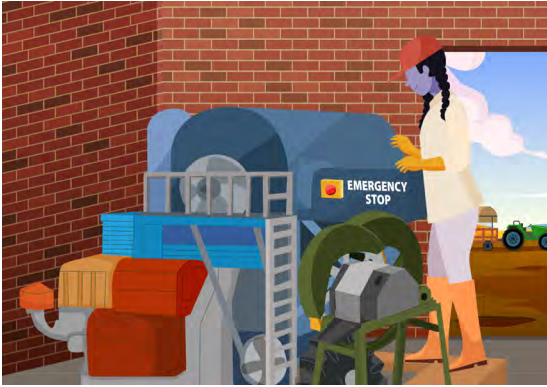
► Figure 15a. Red emergency stop button – large and clearly visible and easy to reach
