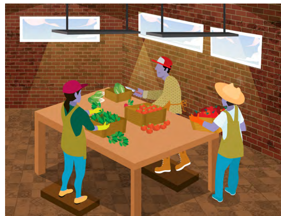
► Figure 18d. Combined use of artificial light and daylight when daylight is insufficient
