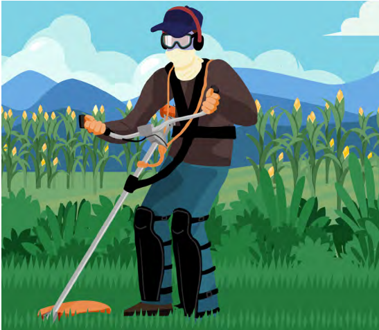
► Figure 10a. Manual mowing machine with strong, firm handles for safe work
