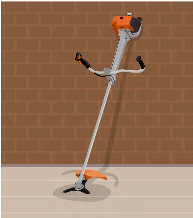
► Figure 13b. Special safety guard on a hand tool to prevent accidents and injuries to operators and people nearby
