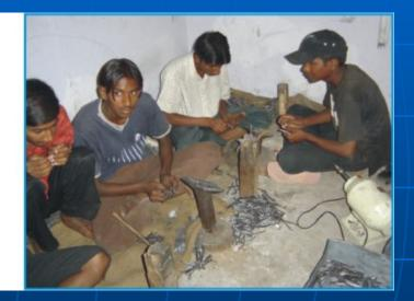
Providing guards on the grinders, introducing work clothes and a low bench for sitting
