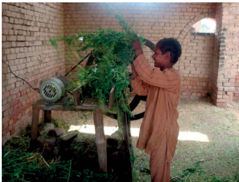
Fodder is pushed by hands into the fodder chopper creating risks of severe injuries.
