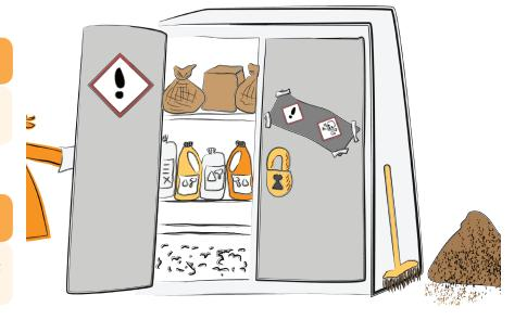
Ensure that any spillage or leakage will be contained in the store. For instance; place a capture tray below the liquids or build a small wall around the store.
