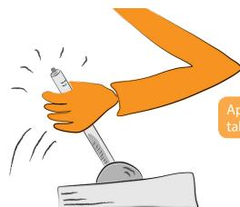
Apply the handbrake to ensure the tractor will not move and take it out of gear.
