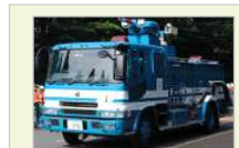
Workers operated this type of water canon to cool the plant at Fukushima
