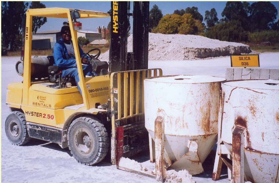
Silica is transported in holders to be deposited into tanks for the production process.
