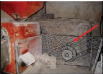
III. USE FEEDING AND EJECTION DEVICES TO INCREASE PRODUCTIVITY AND REDUCE MACHINE HAZARDS.
