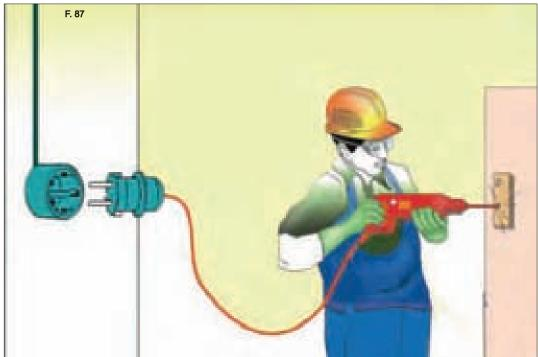
Figure 87: Use appropriate electrical plugs with earthed correctly.
