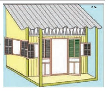
Figure 88: Open more windows and doors, remove obstacles that prevent natural ventilation.
