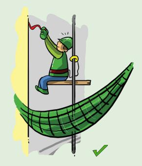
360° protection is required at all work areas where there is a risk of falling. This is achieved by double guard rails, toe-boards and ensuring a minimum gap between the working platforms and any structure. Safety netting and safety harnesses can also be used to enhance safety. However these do not prevent a fall but mitigate the consequences of the fall.
