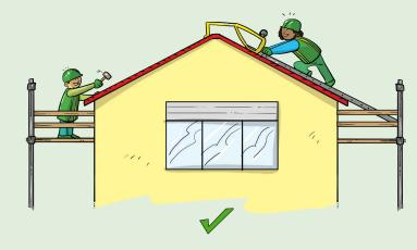
Control measures to prevent workers from falling may include an upper guard rail at approximately 1 meter and an intermediate guard rail at a height of approximately 0.5 meter above the working platform. A toe board should also be present to prevent objects falling on to persons below.
