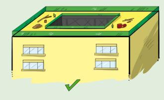
Wherever guard-rails and toe-boards cannot be provided alternative measures are required, for example safety nets or safety harnesses attached to secure anchor points.
