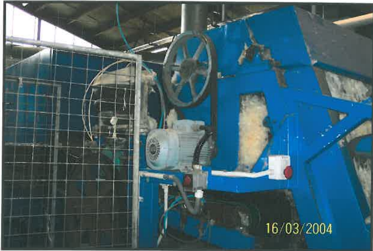
Photo 3 - Unguarded Chain & Sprocket Transmission
