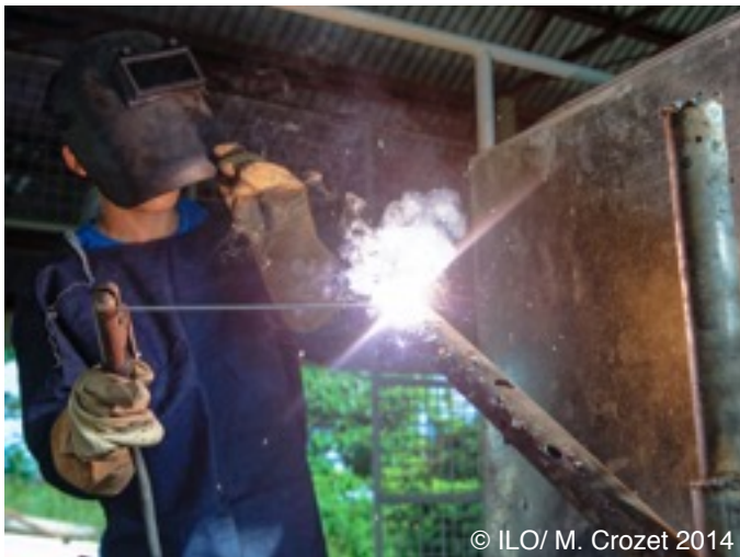
A trainee demonstrates his newly acquired skill in shielded metal arc welding (SMAW).
