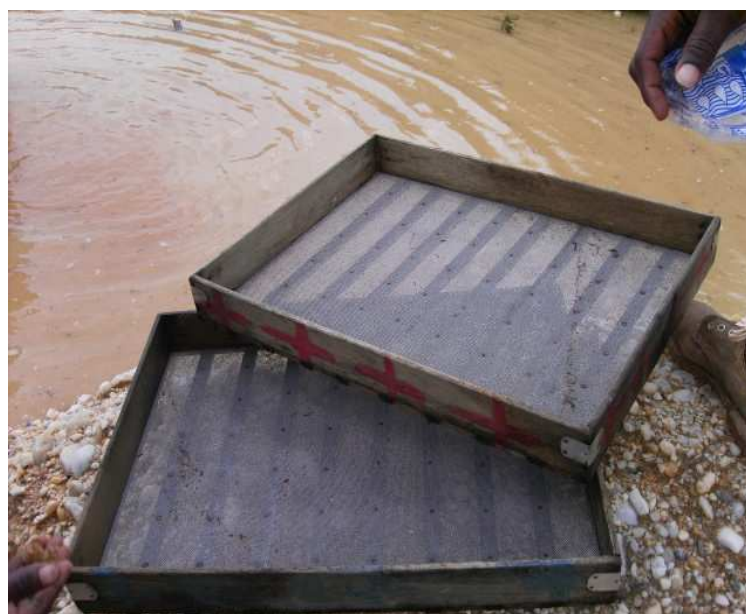
Picture 2: Sieves for separating diamonds-containing stones from ordinary stones
