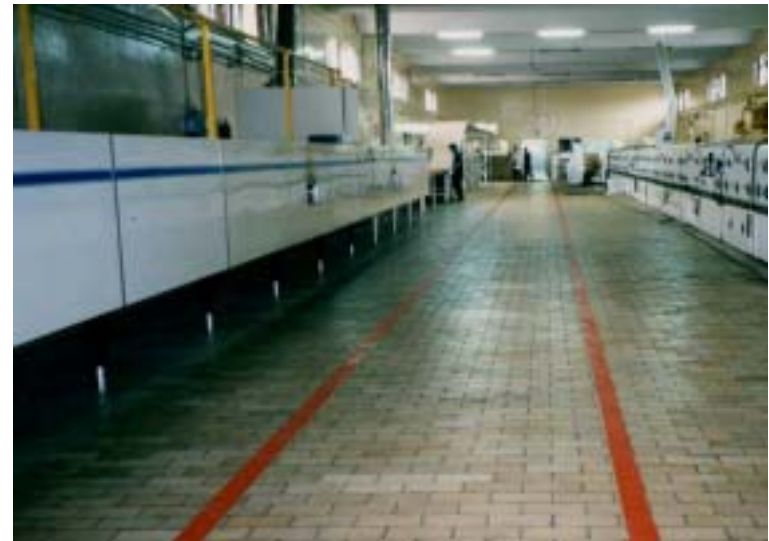
Clear passageway with marker lines.
