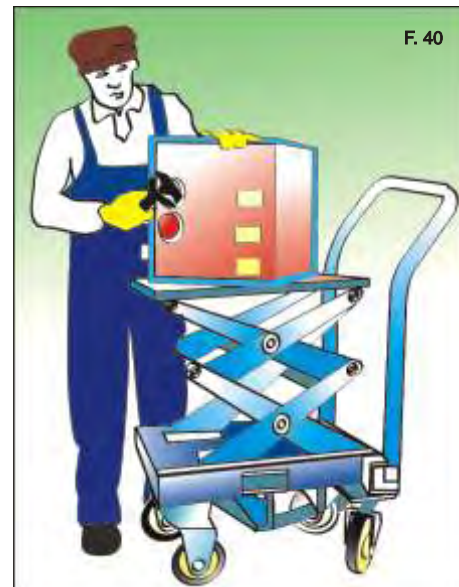
Figure 40: A manually powered device for lifting heavy item to working level.
