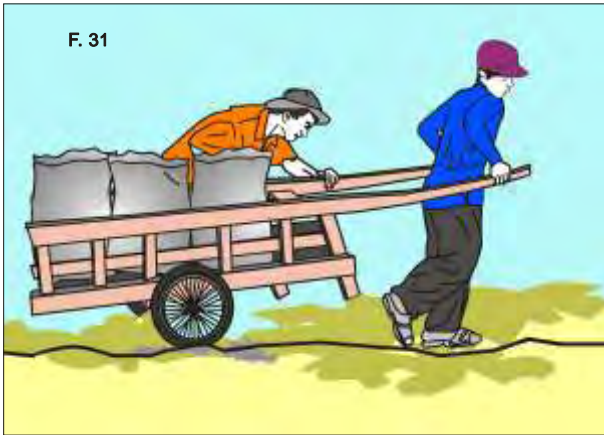
Figure 31, 32 : On rough roads, it is easier to push or pull hand-trucks with big wheels than those with small wheels.
