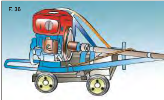
Figure 36: Use a wooden bed with wheels to move heavy agromachinery.
