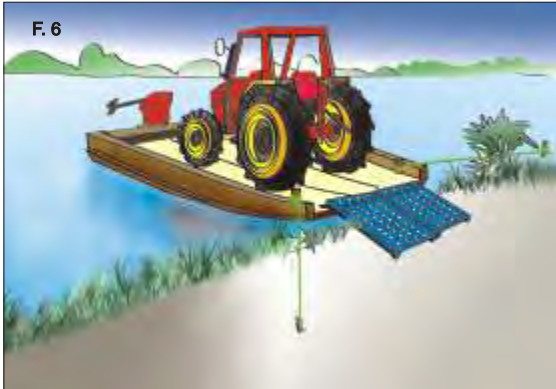
Figure 6: Use a sloped platform at the heaps of earth or rough field edges.
