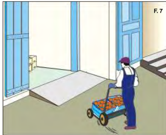
Figure 7: Provide ramps with a small inclination over stairways for easier pushing of carts or wheeled racks.
