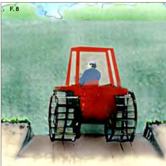
Figure 8: Provide sloped form in the rice field for the smooth movement of agro vehicles.
