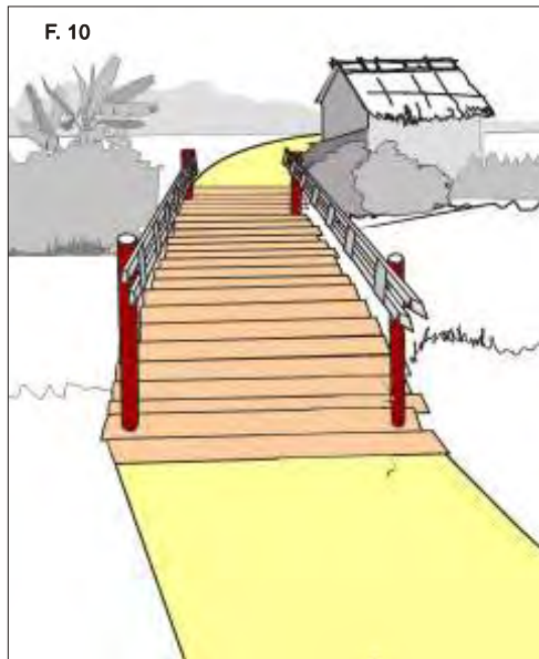
Figure 10: Wooden bridge with firm handholds constructed over stream. Bridge bed is wide enough, for the transport of people and farm products.
